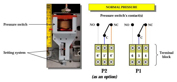
When the tank pressure reaches the set-point value ( $\pm 0.01$  bar), the pressure switch's contact changes position.
